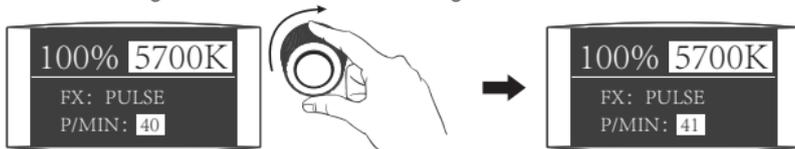
Rotate the "right knob" and set the P/MIN.
