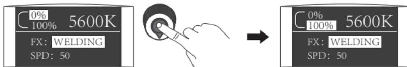
Press in the "left knob" to select DIM1, DIM2, CCT.
