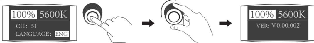
Rotate the "right knob" then you can check the current version for the fixture.
