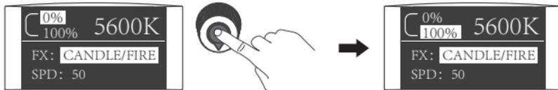
Press in the "left knob" to select DIM1, DIM2 and CCT.
