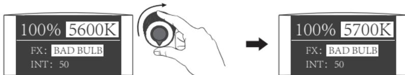
Rotate the "left knob" to set the parameters.
