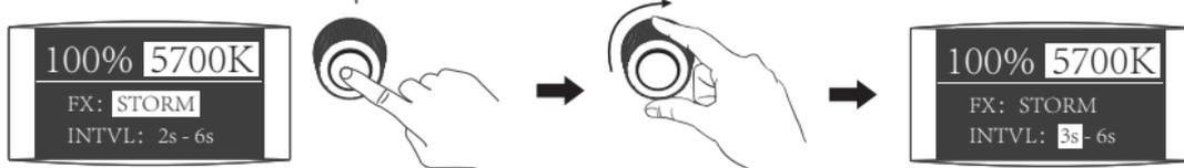
Press in the "right knob" to enter INTVL range setting, then rotate it to set the INTVL range.
