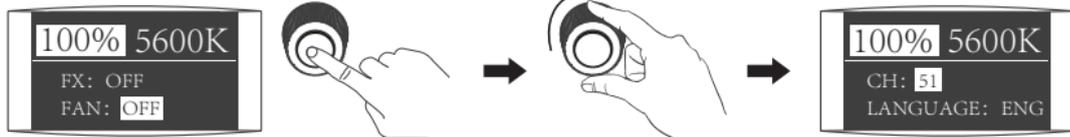
Press in the "right knob" to enter CH setting, then rotate it to set the address code for the fixture.
